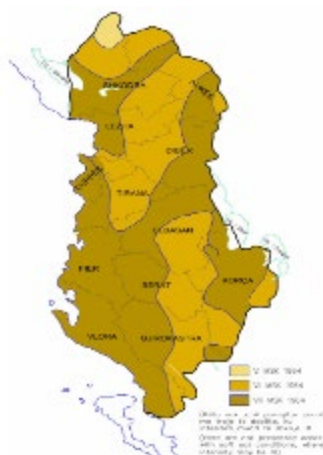
Figure 74: Map of S_a(0.2) 5 % damping for Albania on rock site and for probability 10 % / 50 years or 475 years return period (Left) and the Map of Seismic Hazard in Albania (Right) (Source: Aliaj et al. 2010).
