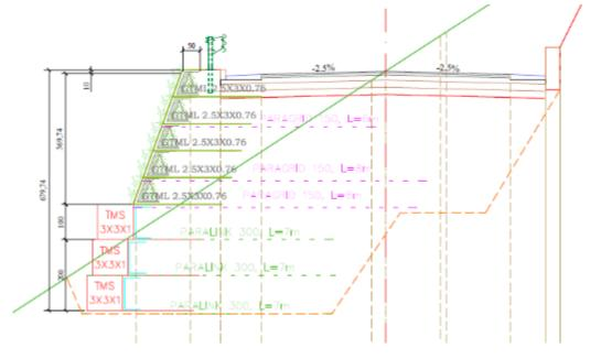
Figure 2.12: Section view of road with scaled embankment
