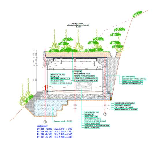
Figure 2.13: Section view of an open sided tunnel on steep sloping terrain
